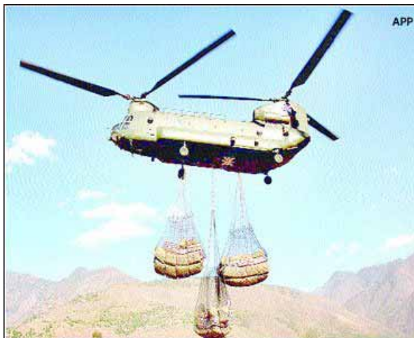
DFID/RAF Chinook CH-47 with underslung load heading to the Neelum Valley from Muzaffarabad. The underslinging allows faster turnaround and more sorties.
